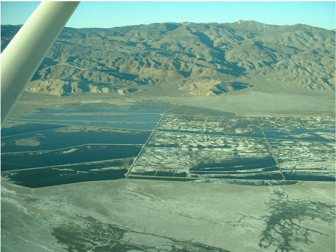
Figure 5.5 – Shallow Flooding – aerial view of pond flood method (left side of photo)
