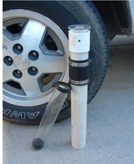
Figure 2.3 - Example of a Cox Sand Catcher (CSC) with the inner sampling collection tube removed.
